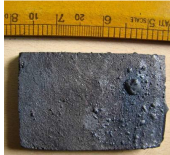
Fig. 6.5 Representative photo of the SiC ceramic composite sample synthesized from coir fibreboard bio-precursor
