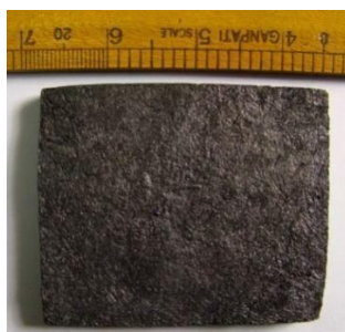
Fig. 5.5 Photograph of a carbon template sample showing no major distortion in shape
