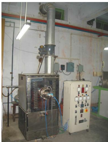
Fig. 5.4 Photograph of the pyrolysis set-up used for carbon template making
