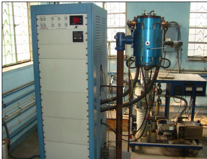
Fig. 6.4 Photograph of the controlled atmosphere/vacuum furnace facility of CSIR-CGCRI used for RLSI processing of SiC ceramic composites from coir fibreboard bio-precursors
